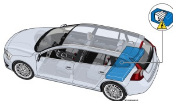
Figure 2. Batteries ensemble location
